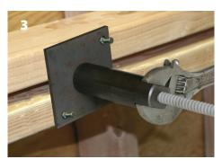
Lock the Form Fixture onto the fiberglass rod by turning the "Form Fixture" clockwise.
