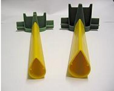
The crack inducer grid used in Australia is a one meter square grid comprising extruded plastic tubes and plastic four-way junctions. The plastic tubes are supplied cut to length for the one meter square grid, and the grid is assembled on site with the tubes fitting snugly onto the junctions.
